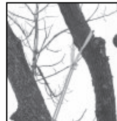
Friction saver shown installed in tree.
