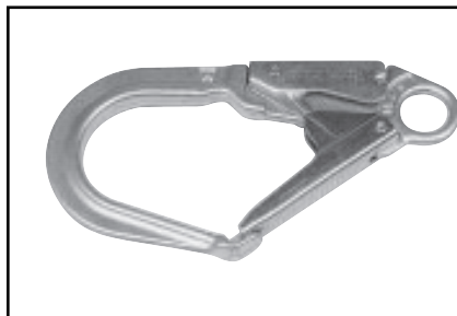
3130 Large Locking Ladder Snap (Option R) 1" eye (I.D.) 2.500" opening 9 3/4" length 1 lb. 8 oz. weight Rated to 5,000 pounds
