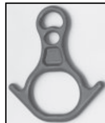
3130 Large Locking Ladder Snap (Option R) 1" eye (I.D.) 2.500" opening 9 3/4" length 1 lb. 8 oz. weight Rated to 5,000 pounds
