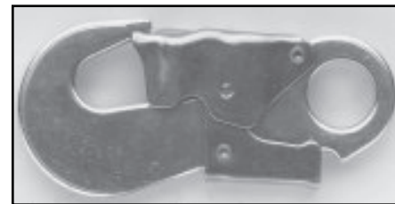
1708 Aluminum Body Locking Rope Snap Hook (Option +6) 7/8" eye (I.D.) .718" opening 5 1/4" length 5.4 oz. weight Rated to 5,600 pounds
