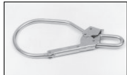
3034 (Option B) Large Locking Rebar Hook 15/16" eye (I.D.) 3 11/32" opening 13" length Rated to 3968 lbs. (Only to be used on shock absorbing style lanyards)
