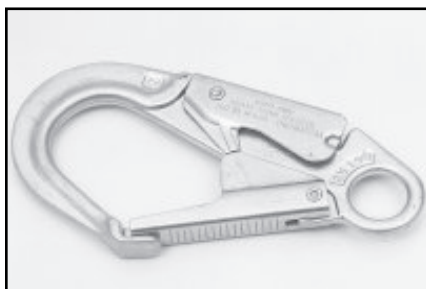
3129 Small Locking Ladder Snap (Option Z) 1" eye (I.D.) 1.750" opening 8 1/8" length 1 lb. 3 oz. weight Rated to 5,000 pounds
